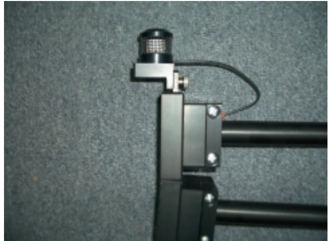
The emitter of airborne ultrasound to be placed above the center of the emitting or receiving probes, said probes to be oriented coincidentally
