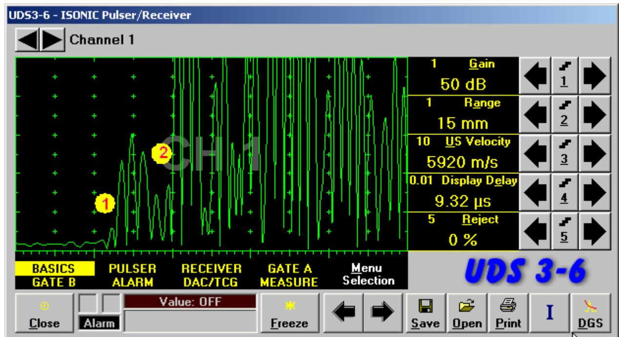
**US Velocity** setting is suitable for steel and thickness of steel layer may be found through direct reading upon placing **Gate A** above signal 1:
