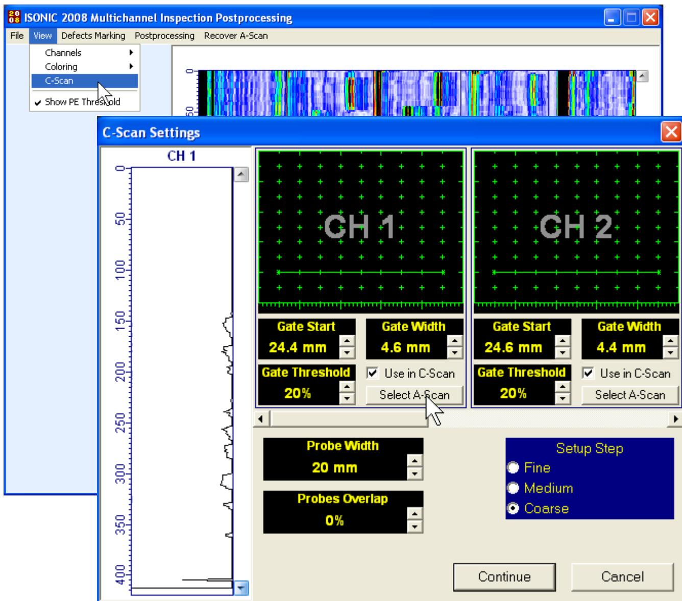
This causes appearance of **C-Scan Settings** screen requiring performing of several preparations. For each strip it is necessary:
