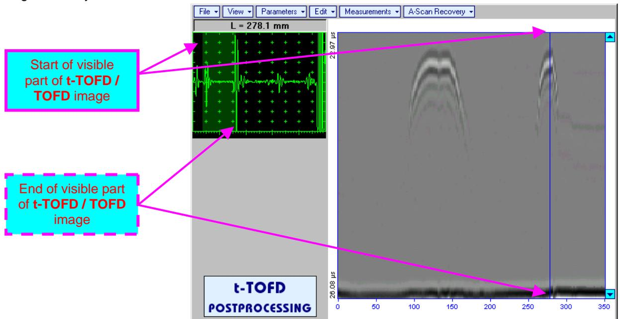
Segment of recovered **A-Scan** corresponding to visible part of **t-TOFD / TOFD** image may be expanded through double click on it – whole **A-Scan** background is green for the expanded segment. Vertical scrolling of **t-TOFD / TOFD** image causes appropriate varying of **Display Delay** for recovered **A-Scan**
