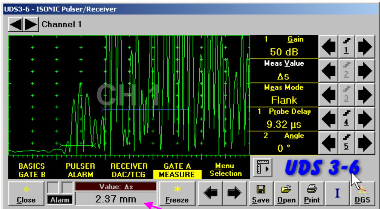
This digital readout was obtained through use of steel **US Velocity** setting (first material) and may not be recognized as a thickness of brass alloy layer (second material)
