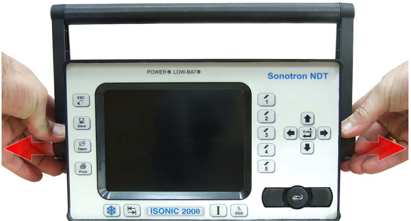
Lift-up and remove the handle:
