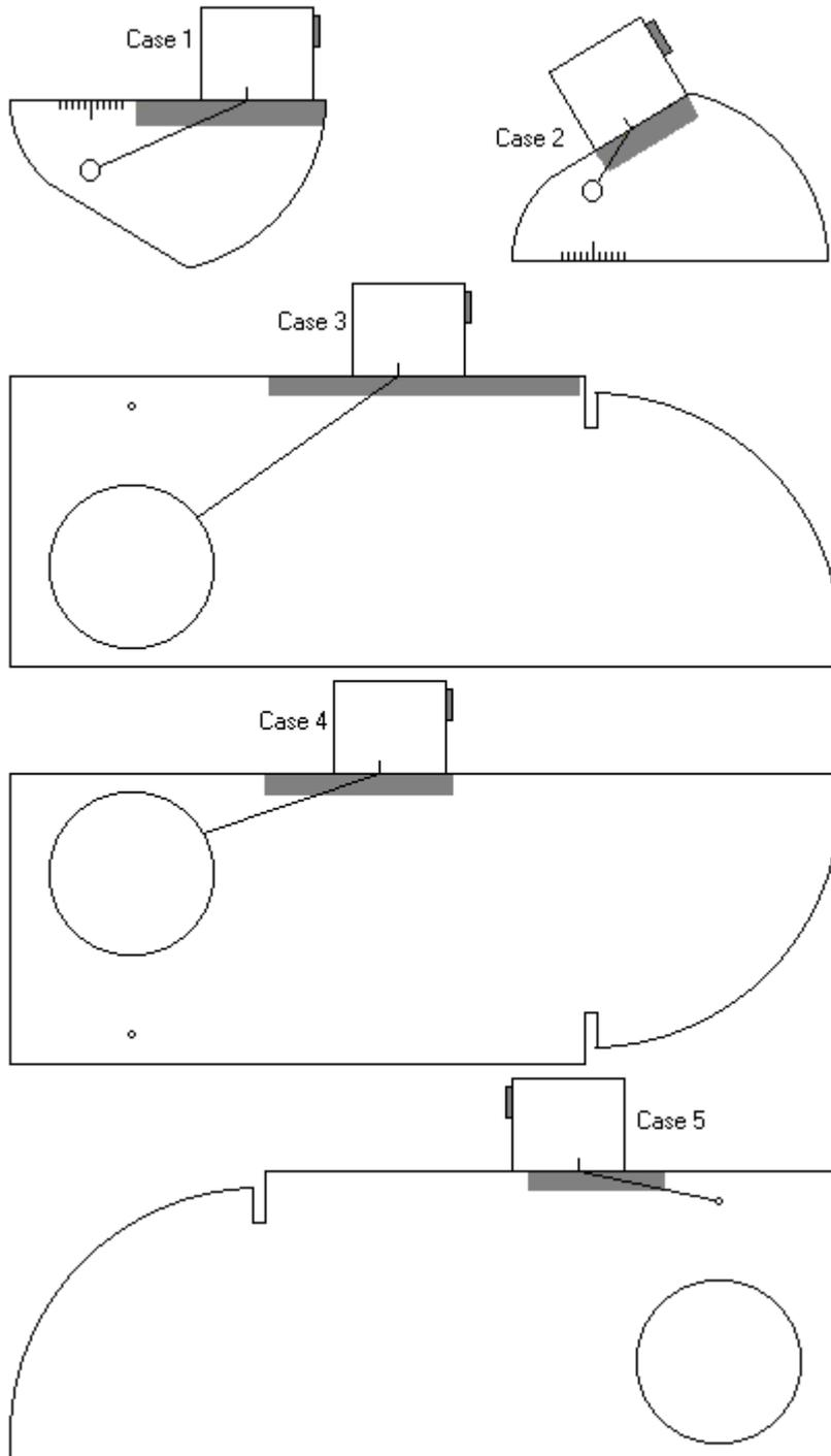
Determining of incidence angle is based on maximizing echo from side-drilled hole in reference block and reading the value of angle from corresponding scale. Depending on probe dimensions and angles there are various reference blocks and scales applicable:
