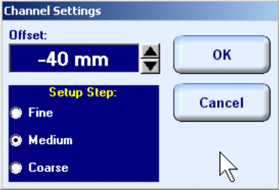
Increment for setting **Offset** value may be selected through check of appropriate option **Fine**, **Medium**, or **Coarse**. To vary **Offset** value click on or press on front panel keyboard or on external keyboard
