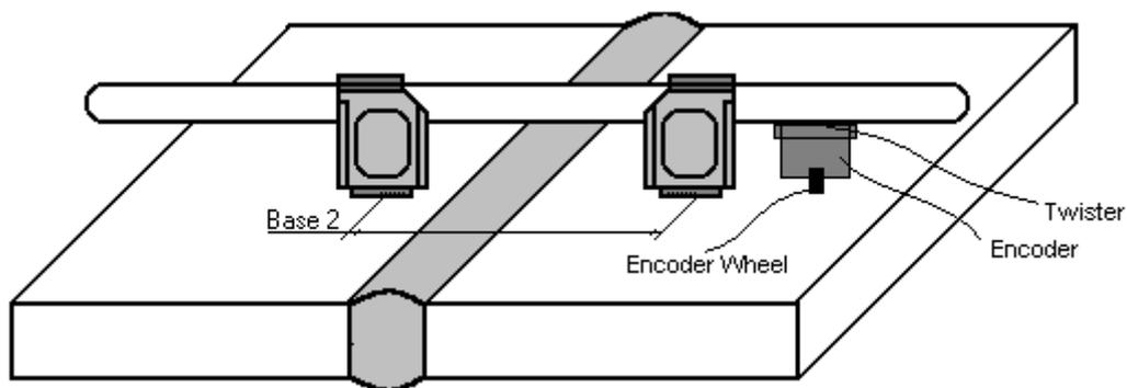
**TOFD** Fixture and encoder positioning for scanning along the weld
