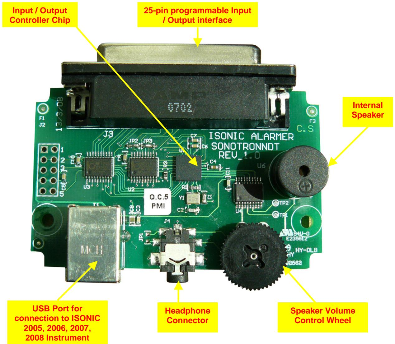
Initially **ISONIC Alarmer** is configured to deliver sound through speaker and headphone connector (standard configuration)
