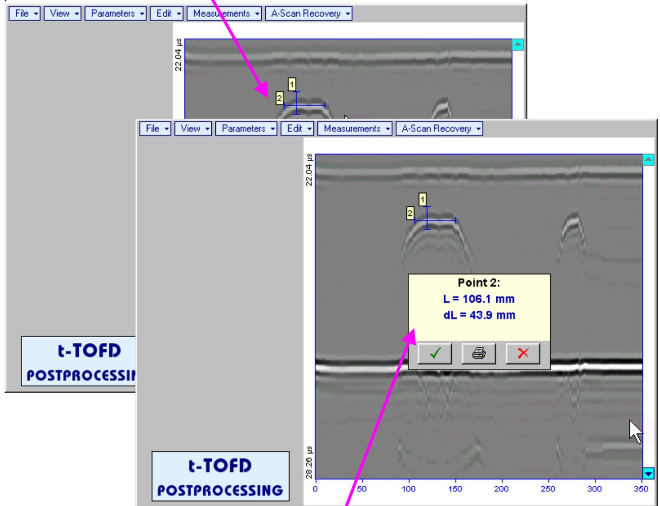
Length measurement results may be recalled into **subwindow** through double click on the *length measurement mark*
