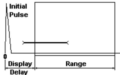
$$SRD = \frac{DisplayDelay}{2} \times USVelocity$$
