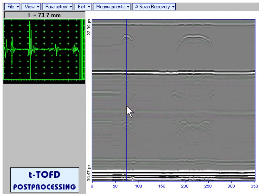
To fix position of *A-Scan base line cursor* with corresponding recovered **A-Scan** left mouse click or release touch screen stylus or press
