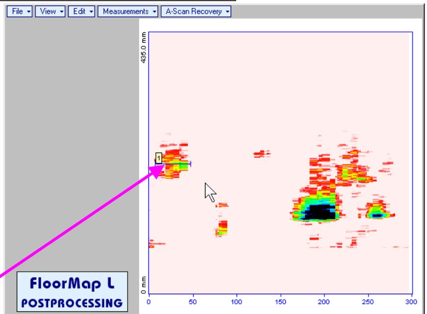
Horizontal **length measurement mark** appears on the **t-FLOORMAP L / FLOORMAP L (CB-Scan)** image upon fixing position of second vertical cursor
