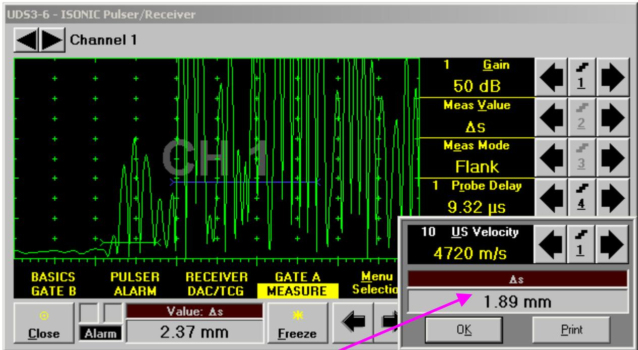
Digital readout for actual thickness of the brass alloy layer (second material) is obtained upon completing setting for second **US Velocity**
