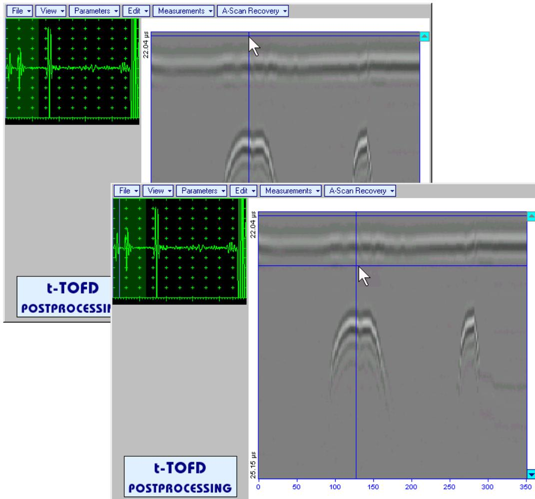
First vertical cursor appears upon designating end of *reference signal*. Its length corresponds to duration of *reference signal* and it is located between first and second horizontal cursors. First vertical cursor may
