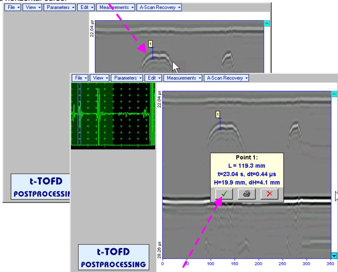
Depth measurement results may be recalled into **subwindow** accompanied with corresponding **A-Scan** through double click on the *depth measurement mark*
