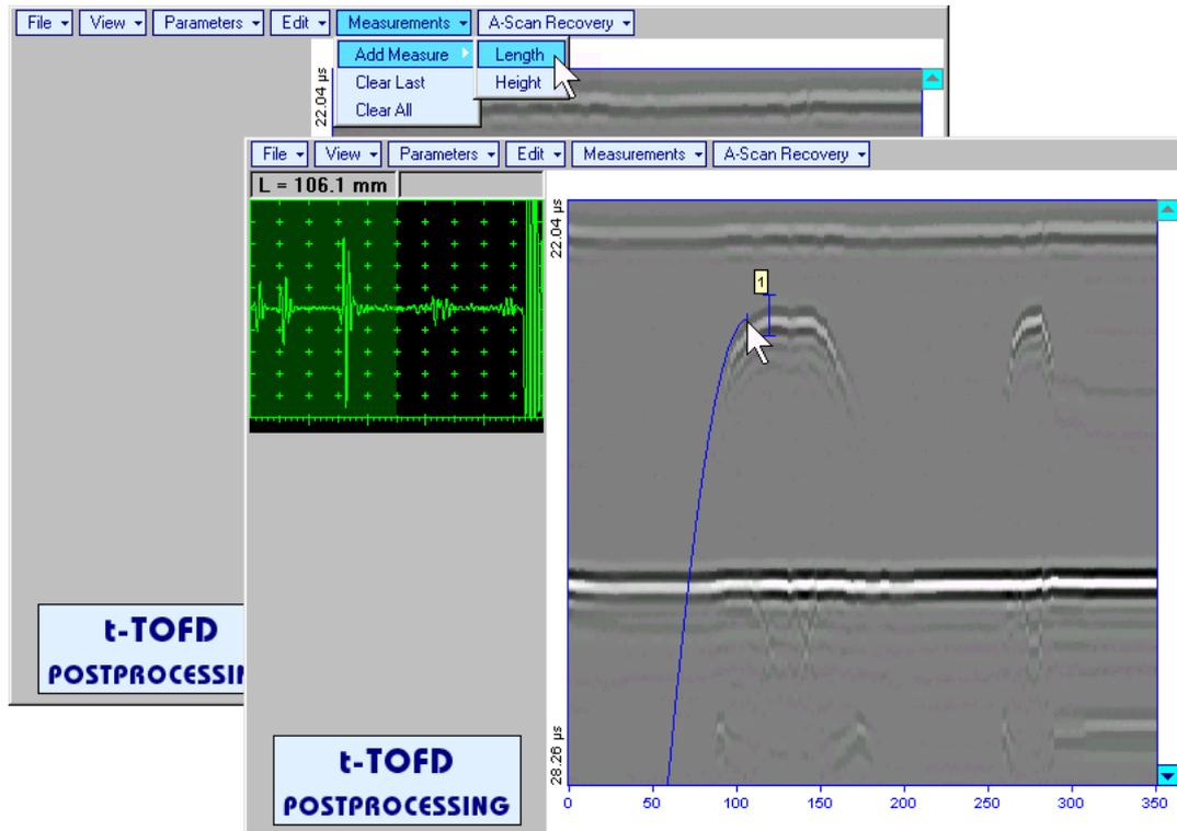
*Right parabolic cursor* appears upon fixing *left parabolic cursor*. It may be manipulated by the same way and must be placed over right defect's end providing shape matching. Coordinate of *right parabolic cursor* along **t-TOFD / TOFD** image measured relatively to position of *left parabolic cursor* (**dL**) is indicated synchronously, it represents length of defect area provided that both parabolic cursors are placed properly
