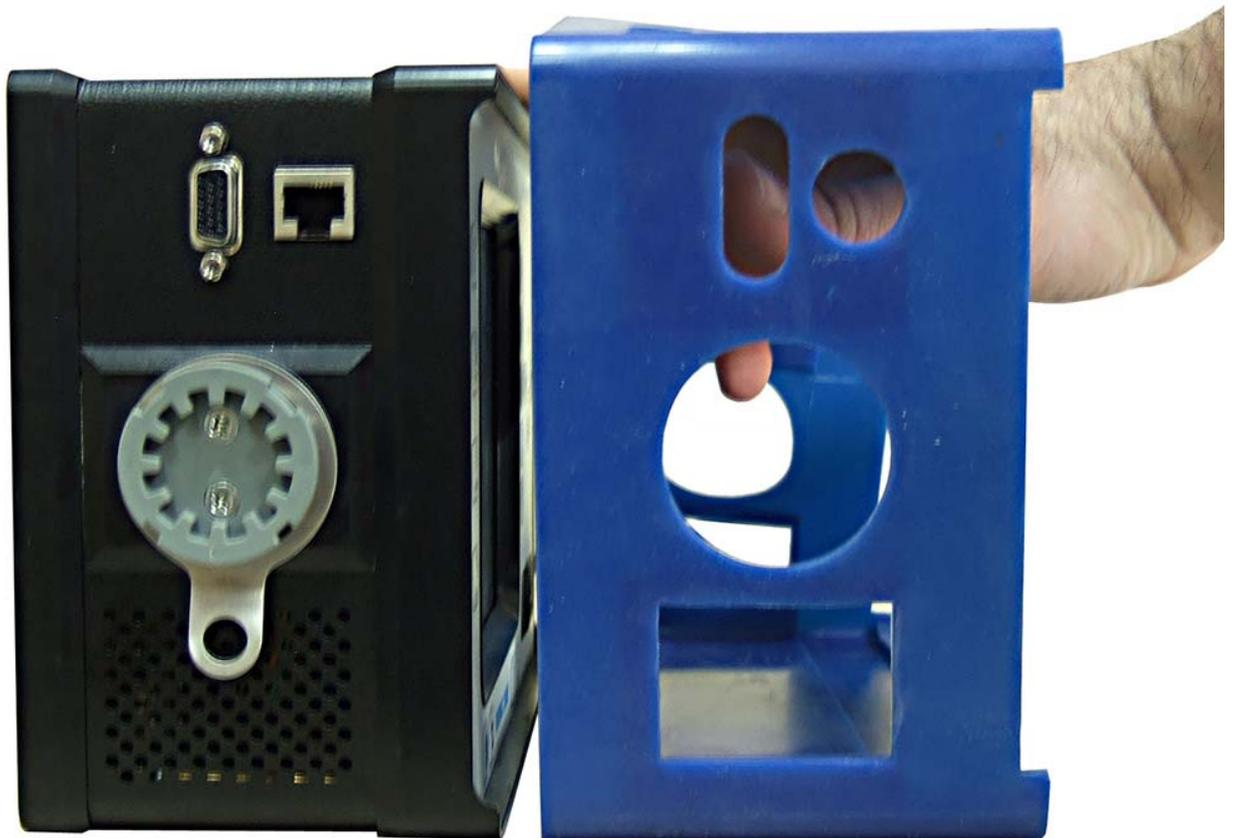
Slip the Silicone Rubber Jacket around the machine until it fits properly and covers all edges:
