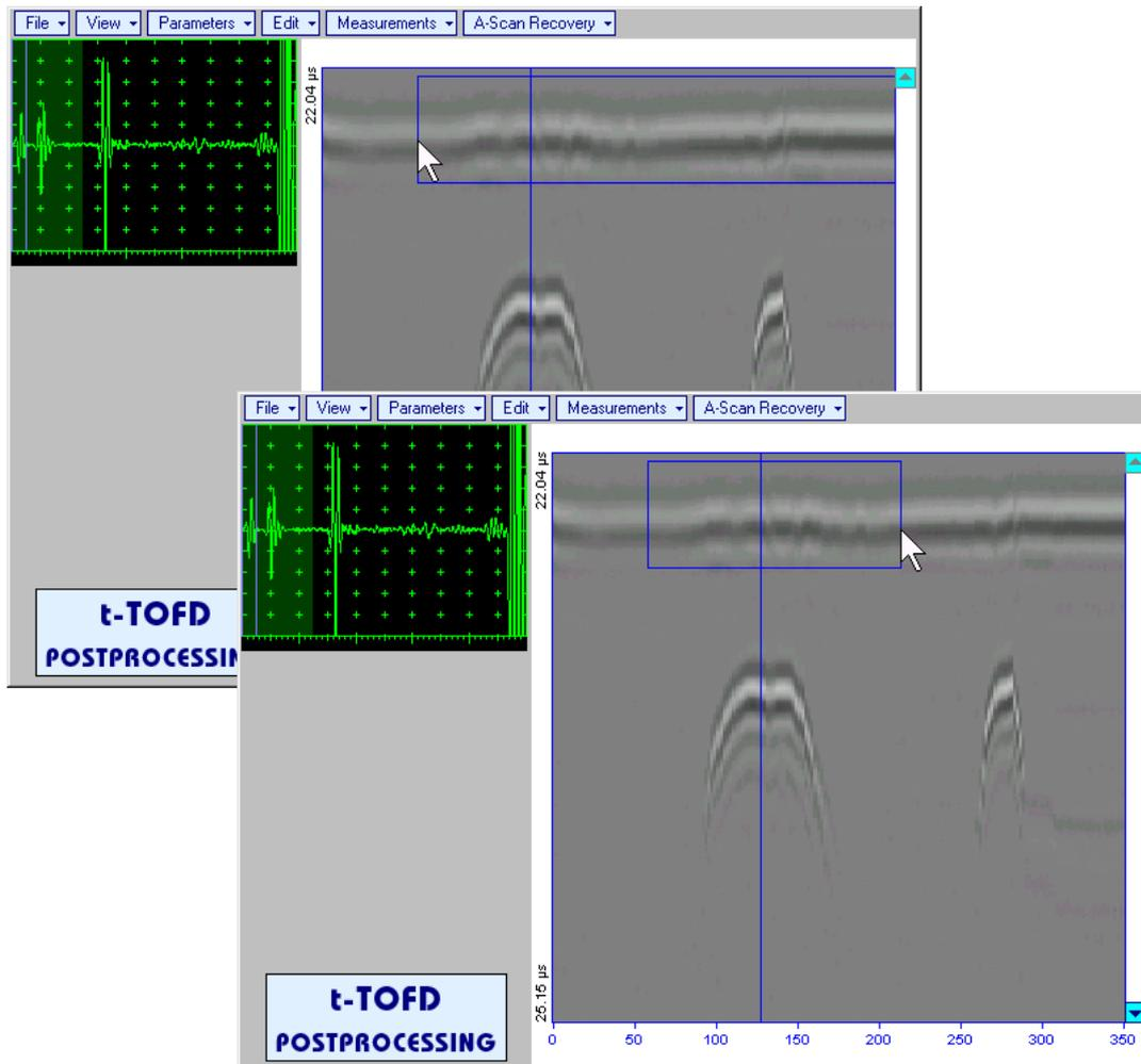
As a result **t-TOFD / TOFD** image is straightened in, above, and under selected *rectangle segment* to compensate deviations caused by various factors during recording, for example, coupling instability, unevenness of scanning or bottom surfaces, etc
