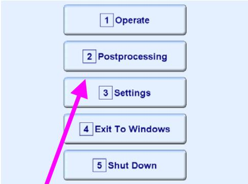
In the **ISONIC 2008 Start Screen** click on **3** or press
