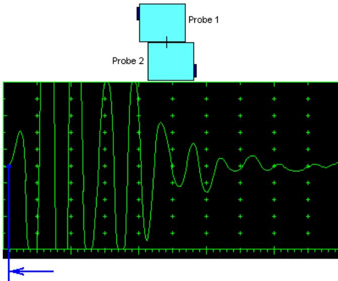
**Stage 4:** Decrease Range to provide ~ 50% of the A-Scan width occupied by the signal
