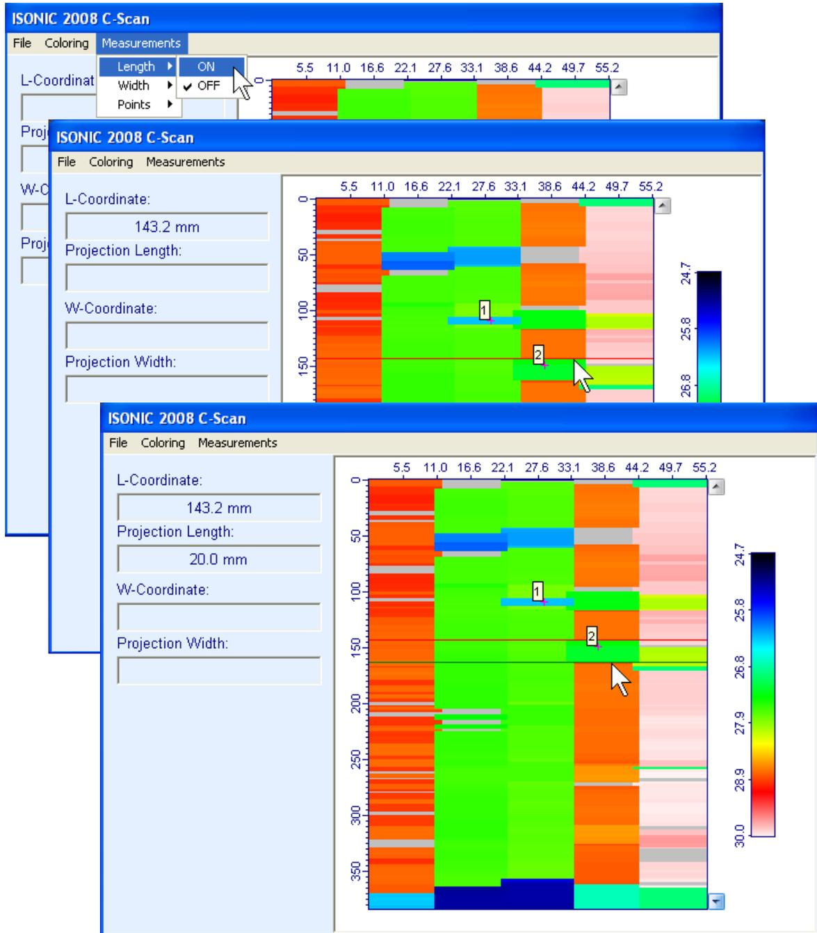
To interrupt **L-Coordinate** and **Projection Length** measurement right mouse click
