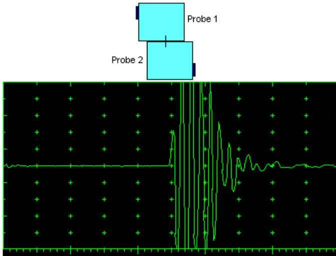
**Stage 3:** Increase Gain to provide height of first half wave of received signal reaching 20 % of total A-Scan height
