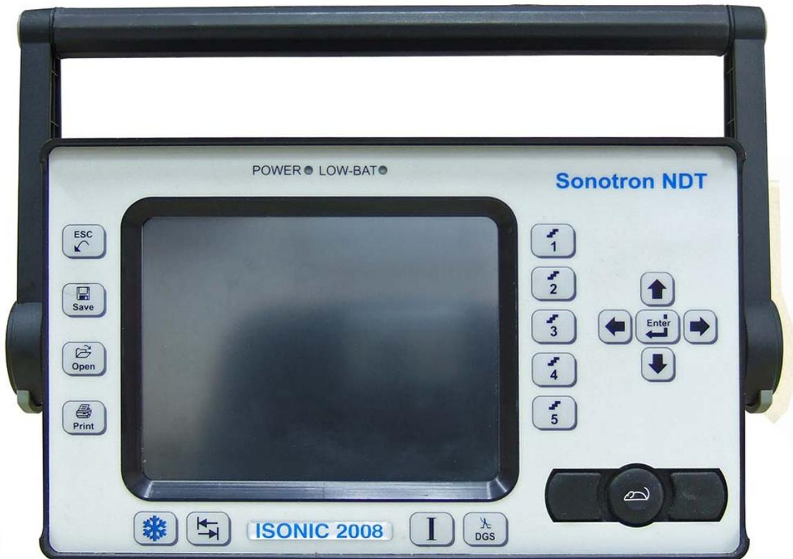
Push the gray buttons of the handle on both sides, and rotate the handle until it is released:
