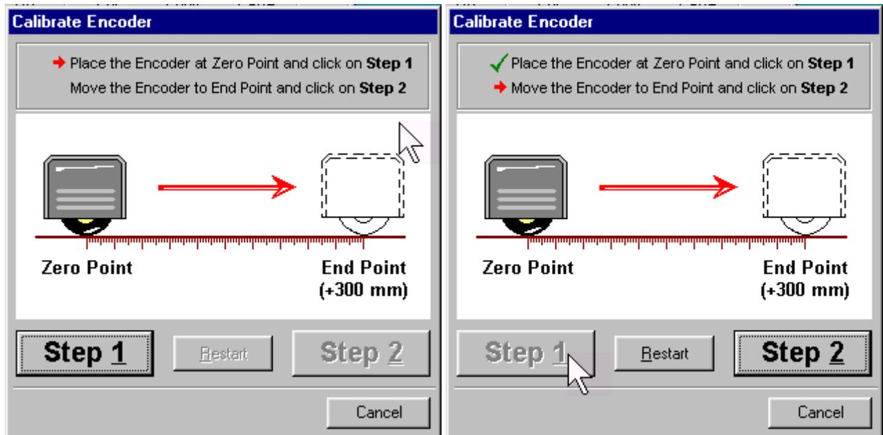
Encoder's wheel while calibrating must pass linearly the distance of **300 mm (12 in)** between **Zero Point** designated through clicking on **Step 1** or pressing **<Alt>+<1>** on external keyboard and **End Point** along scale bar attached to flat surface
