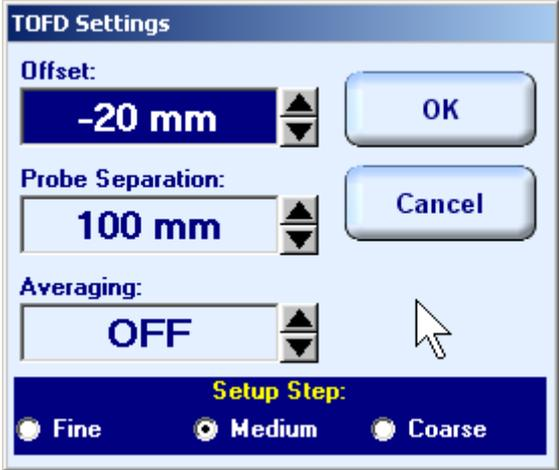
Setting of these values to be performed by the same way. For more data about **Probe Separation** refer to paragraph 6.5.1.4 of this Operating Manual; for **Averaging** refer to paragraph 6.5.2.1 of this Operating Manual
