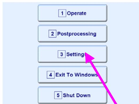
To proceed with the calibration in the **ISONIC 2008 Start Screen** click on **3** or press
