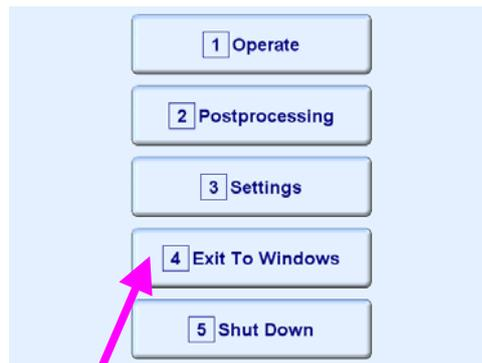
In the **ISONIC 2008 Start Screen** click on **4 Exit To Windows** or press
