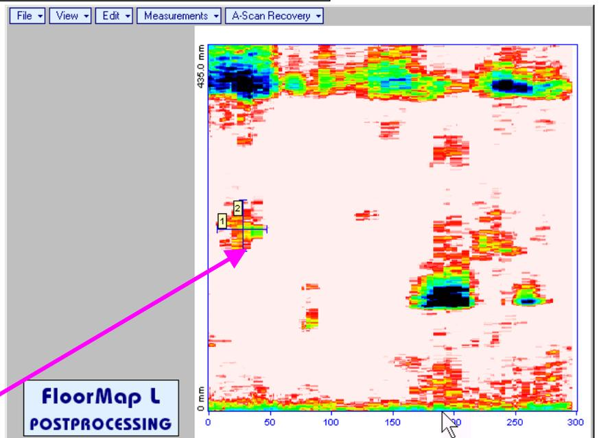
Vertical **width measurement mark** appears on the **t-FLOORMAP L / FLOORMAP L (CB-Scan)** image upon fixing position of second horizontal cursor
