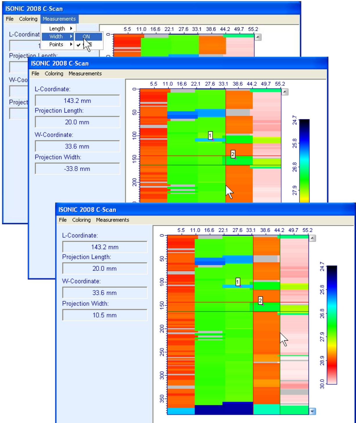
To interrupt **W-Coordinate** and **Projection Width** measurement right mouse click
