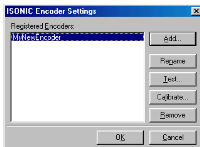
To update the registry of **ISONIC 2008** with new encoder data click on the **OK** or press
