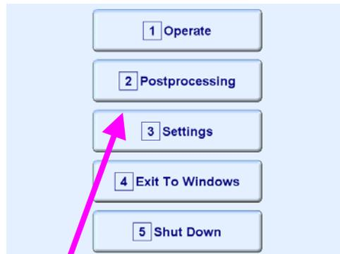
In the **ISONIC 2008 Start Screen** click on **3** or press
