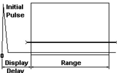
$$SRD = \frac{DisplayDelay}{2} \times USVelocity$$
