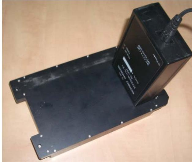
There is **Charge** LED on the charger. While charging the battery this LED emits solid light. **Charge** LED starts flashing upon charge is completed
