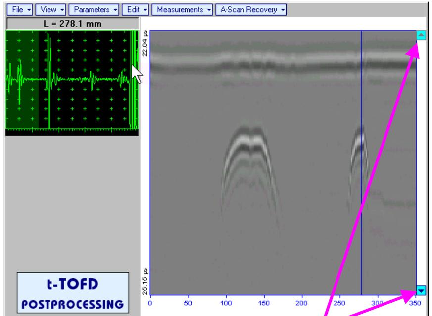
Expanded **t-TOFD / TOFD** image may be scrolled it vertically using appropriate **buttons**
