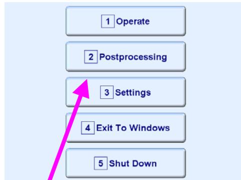
In the **ISONIC 2008 Start Screen** click on **3** or press
