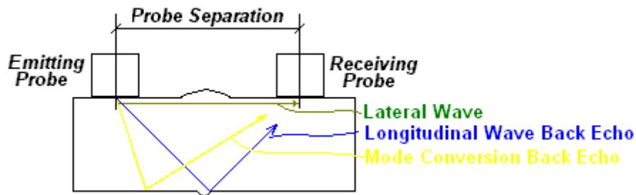
**Probe Separation** should be optimized according to Inspection procedure and probes positions in the TOFD fixture to be fixed upon. **Display Delay** and **Range** to be adjusted then to provide representing of signals according to Inspection procedure – the typical examples are given below for 40 mm thickness welded plates.
