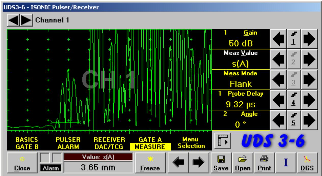
If placing now **Gate B** above signal 2 and selecting  $\Delta$ s as **Meas Value** then interval between signals 1 and 2 will be measured. To obtain proper  $\Delta$ s readout value of **US Velocity** valid for brass alloy layer (second material) must be keyed in
