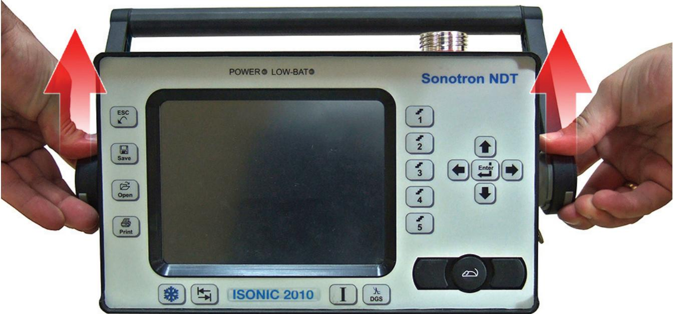
4. Place the Silicone Rubber Jacket so that the holes match the ports of the ISONIC machine:
