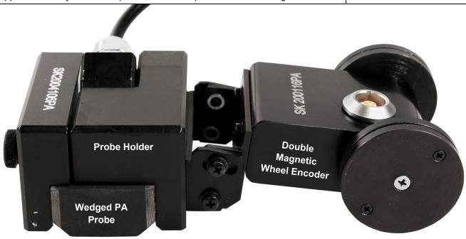
Example of assembly: S 4922214381 equipped with S 4922214702 delay line for the compression wave inspection, scanning, and recording with use of SK 2001116 PA encoder and SK 2004145 PA probe holder
