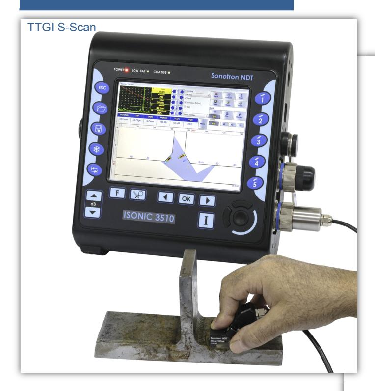
On-the-run toggling between True-to-Geometry Imaging (TTGI) S-Scan and Live FMC/TFM
