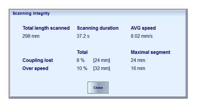
Quantitative Scanning Integrity Report may be generated automatically as soon as scanning completed. Alternatively thanks to 100% raw data capturing it may be formed out of the stored files at the postprocessing stage
