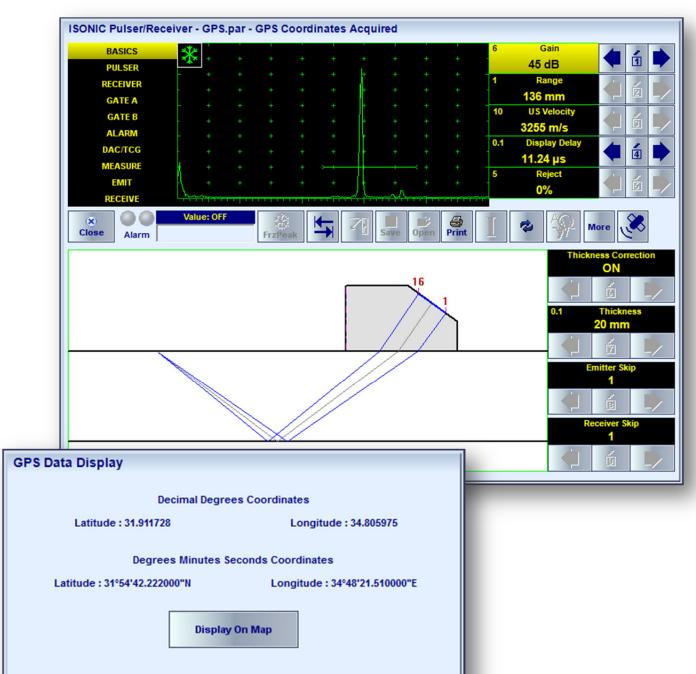
Whilst on the inspection side in the field the GPS coordinate may be obtained and displayed automatically along with UT data with use of an external GPS receiver connected to the instrument's USB Port and embedded into the data files for the reporting purposes
