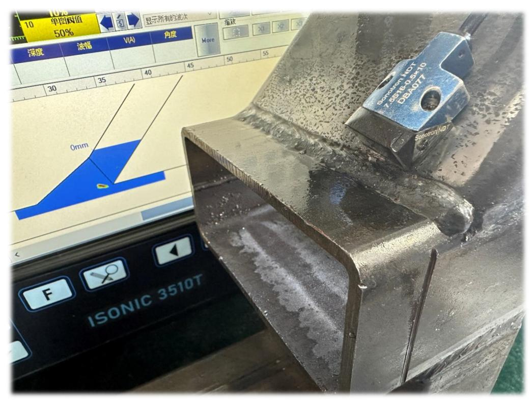
Structural skewed fillet weld between thin wall hollow rectangle profiles
