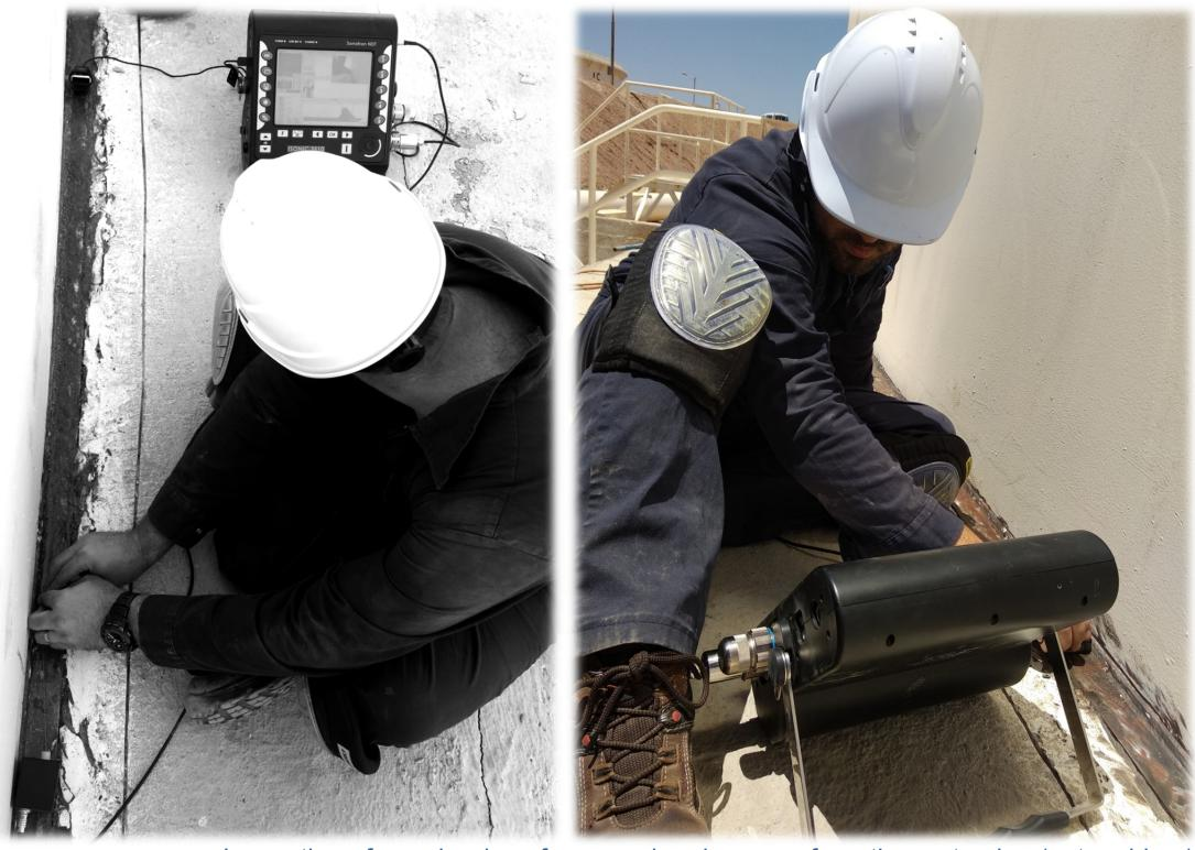
Inspection of annular rings for corrosion damages from the protrusion (outer chime)
