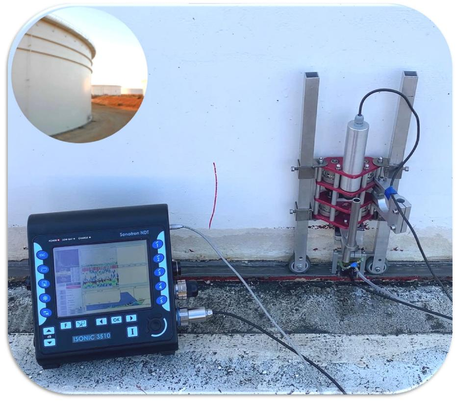
Shear Wave Multiple Skip TTGI S-Scan Coverage - Inspection of the Critical Zone – Automatic Scanning and Recording
