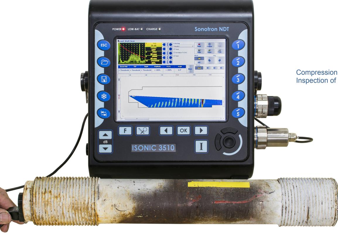
Compression Wave TTGI S-Scan – Inspection of double threaded hollow stud bolt
