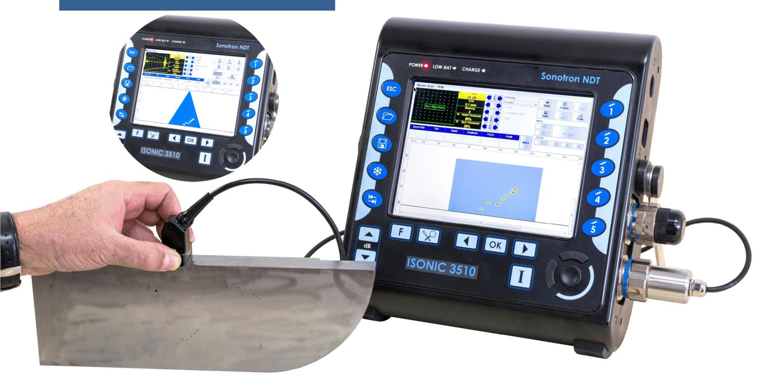
Live FMC/TFM toggled with S-Scan coverage: high sensitivity combined with precise imaging
