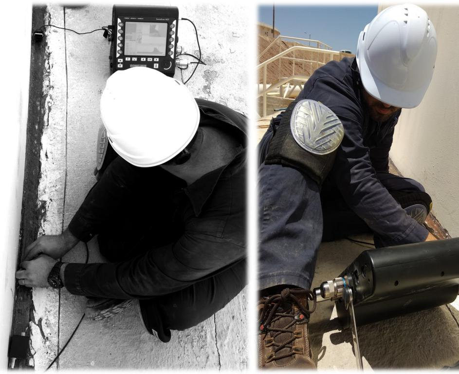
Inspection of annular rings for corrosion damages from the protrusion (outer chime)
