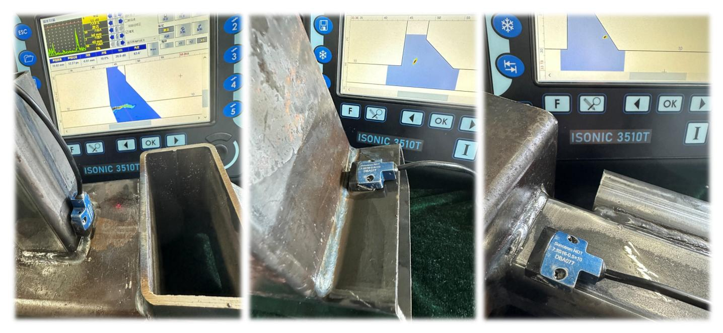
Structural straight corner weld between thin wall hollow rectangle profiles
