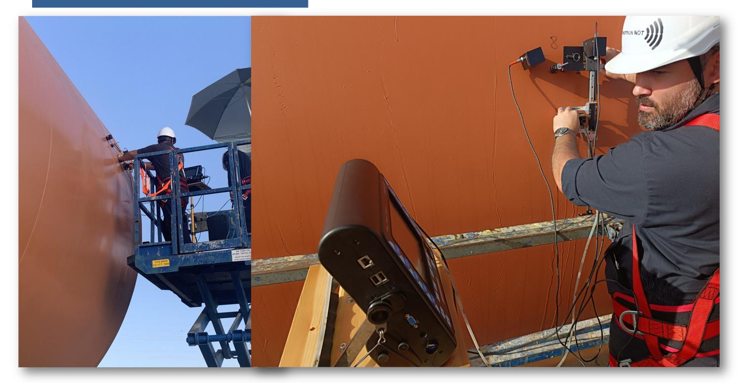
Through Paint / Coating Corrosion Mapping and Flaw Detection
