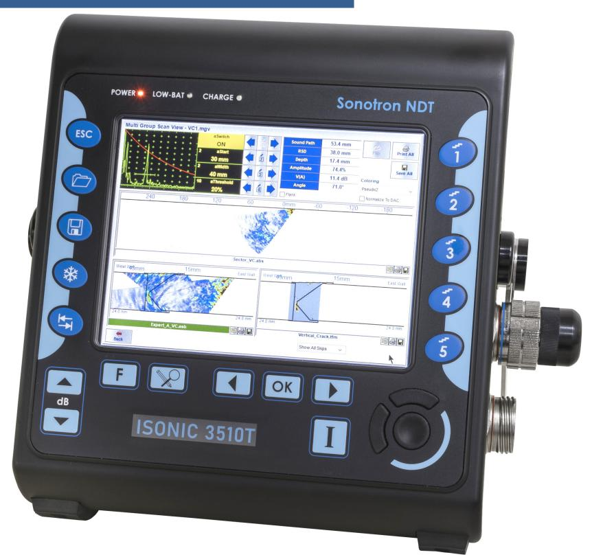
**MULTIGROUP** and **MULTIGROUP** T modes of operation allow implementing of several different scan plans (up to 5) simultaneously out of the same probe increasing the probability of detection and precision of the defects evaluation
