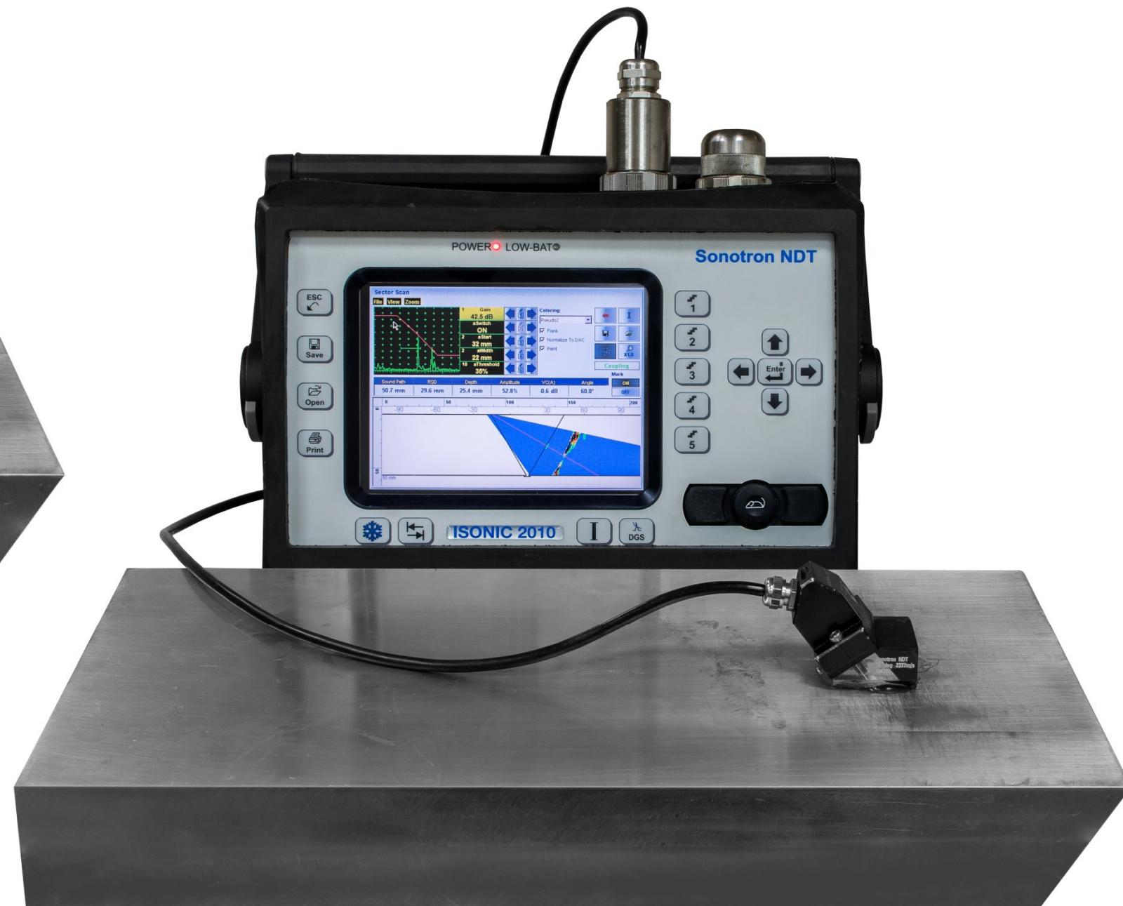
At the first stage the DAC is prepared for the FBH, which is situated at parallel to the weld bevel. For the first present case weld bevel and FBH are is 30 deg inclined
