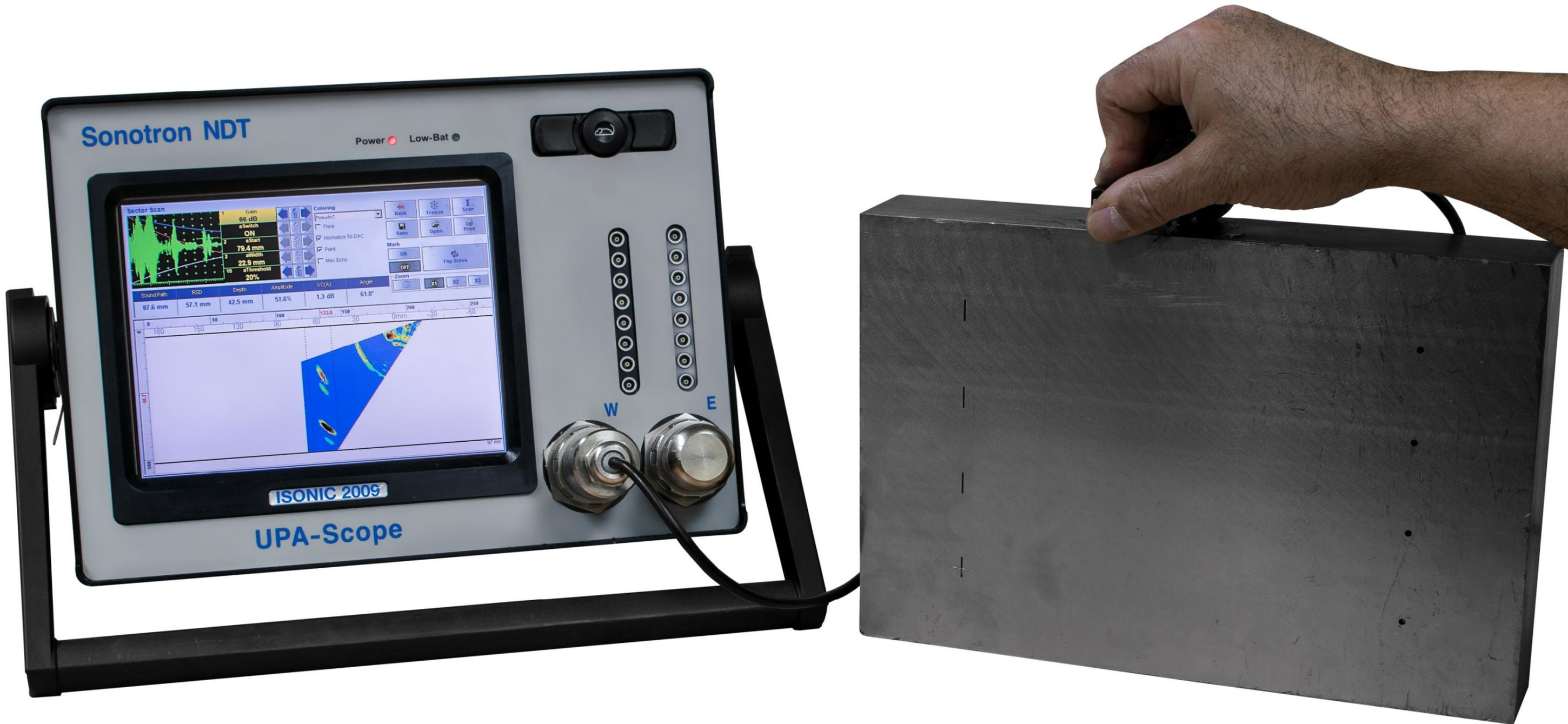
*Reverse TOFD: compression wave PE detection of the cracks and lack of side wall fusion defects in narrow gap heavy thickness welds based on the receiving and waveform analysis of the upper and lower tip-diffraction echoes*
