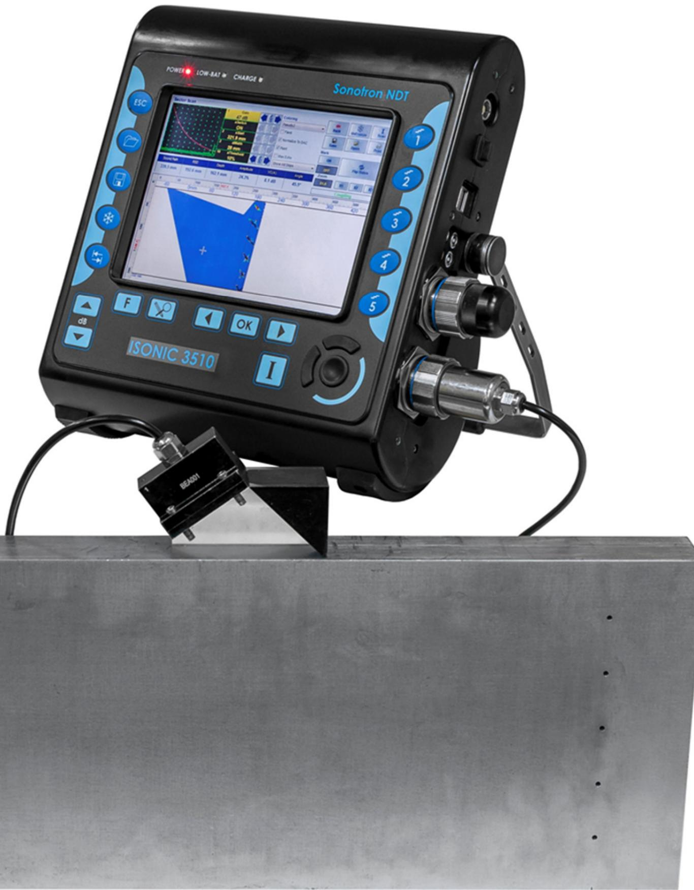
Combined half- and full skip inspection of 200 mm thick calibration block: focal point migrates along the vertical line connecting the centers of the reflectors
