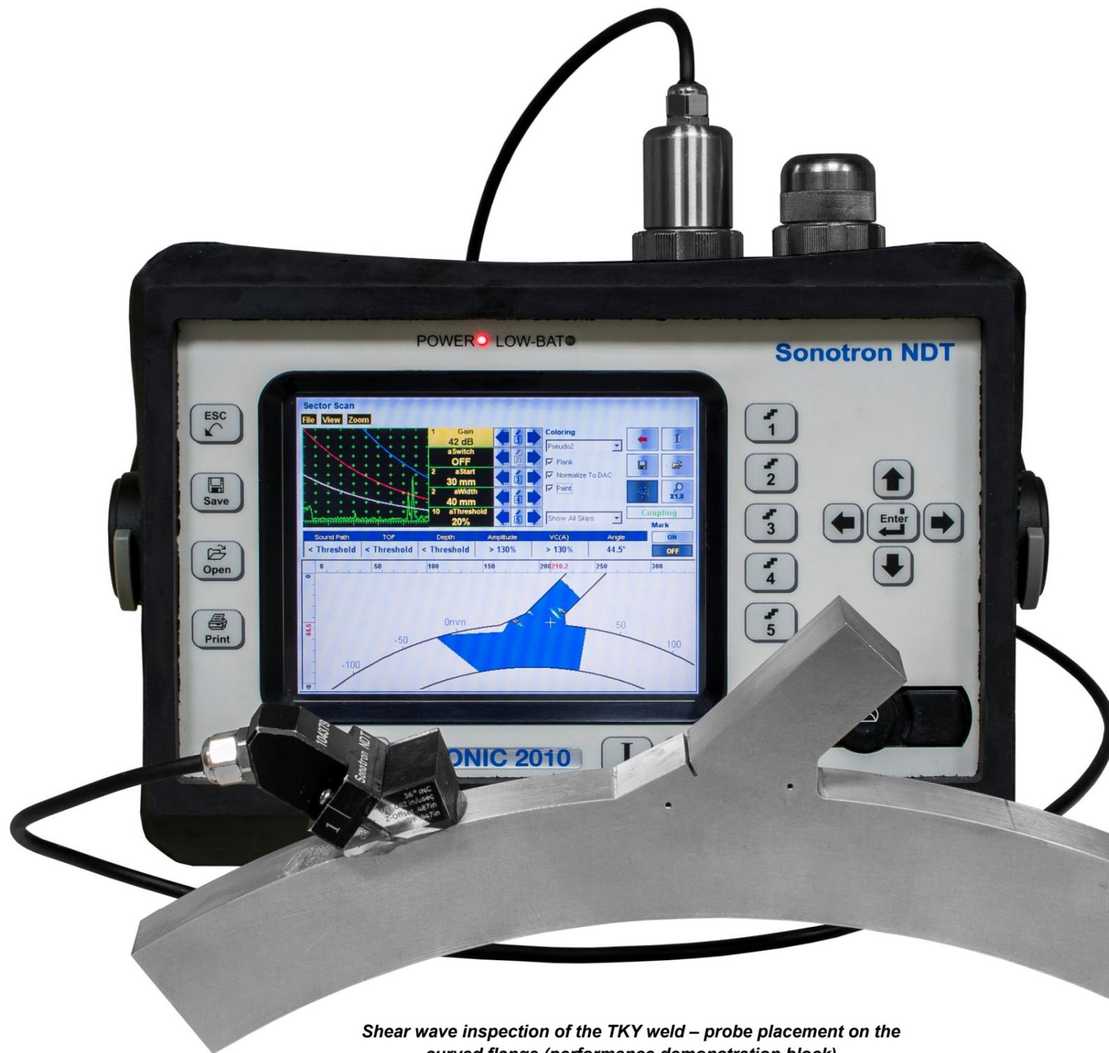
Shear wave inspection of the TKY weld – probe placement on the curved flange (performance demonstration block)
