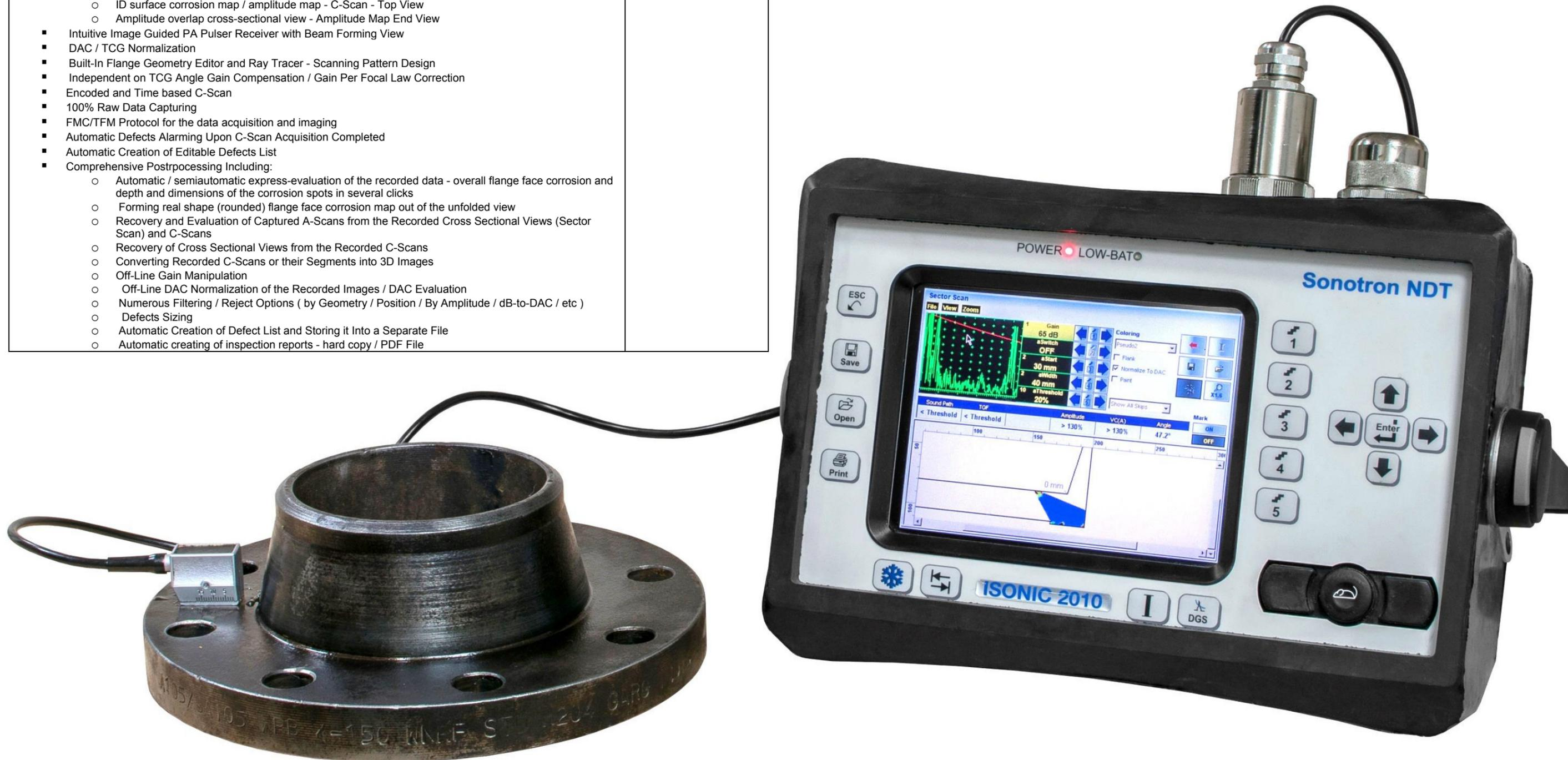
Detection and evaluation of the flange face corrosion
