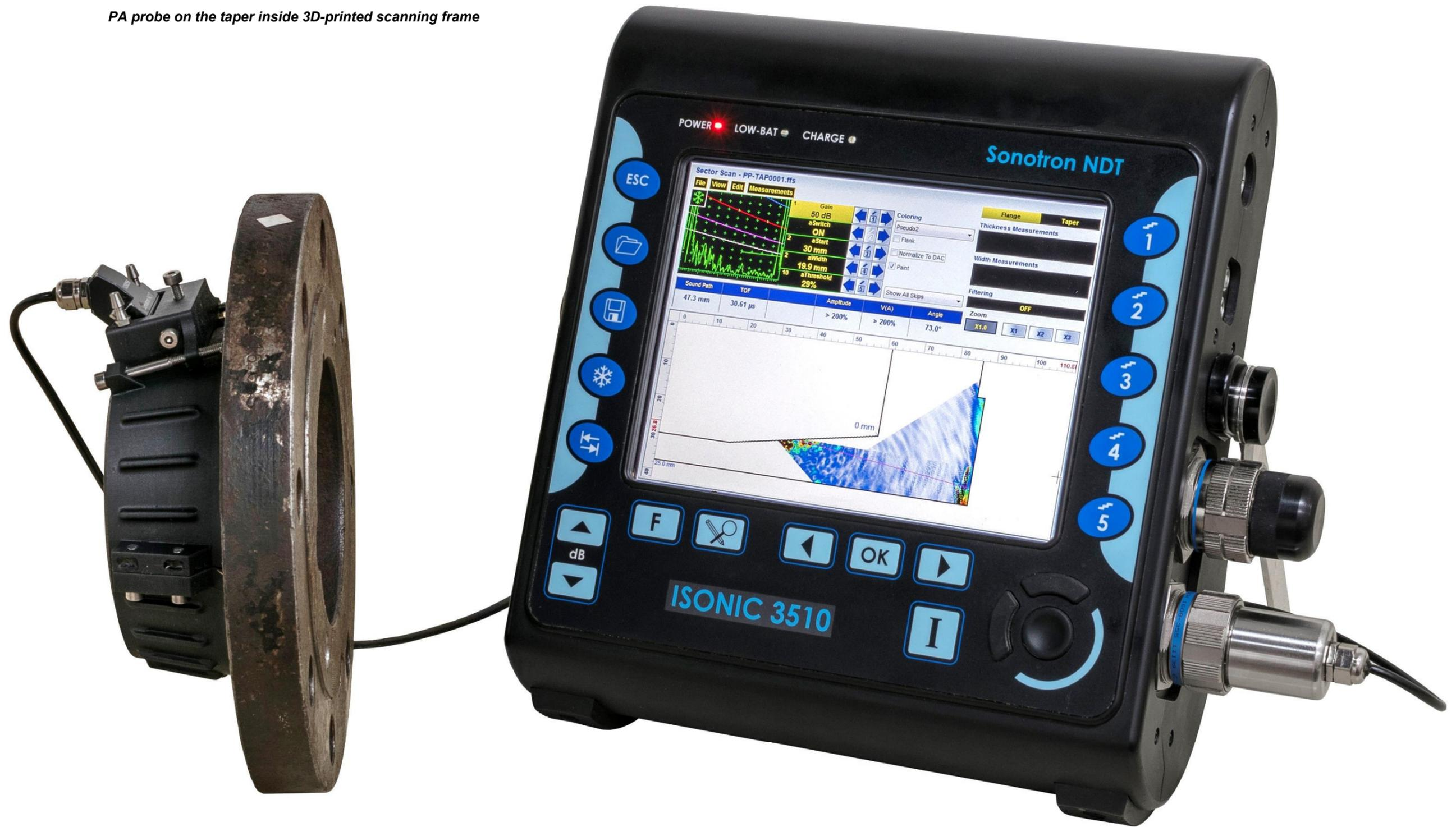
Unfolded map of the material loss on the FFC obtained through the scanning around the taper
