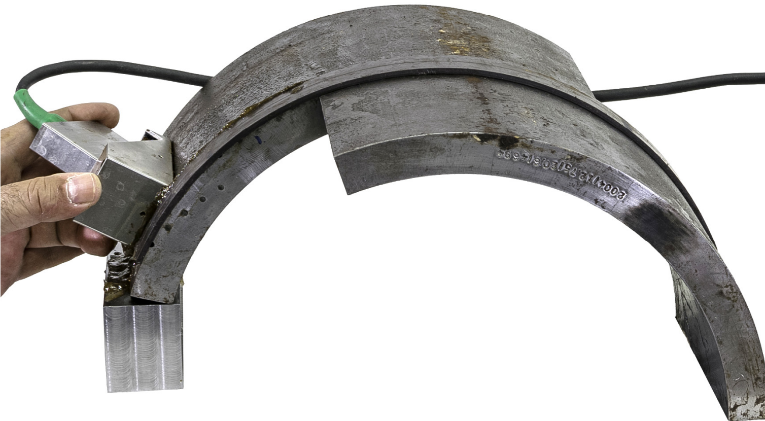
PE strip chart recording through implementing of several Tandem pulsing receiving cycles on Z-cut ASTM E 1961 calibration block for the inspection of narrow bevel girth welds
