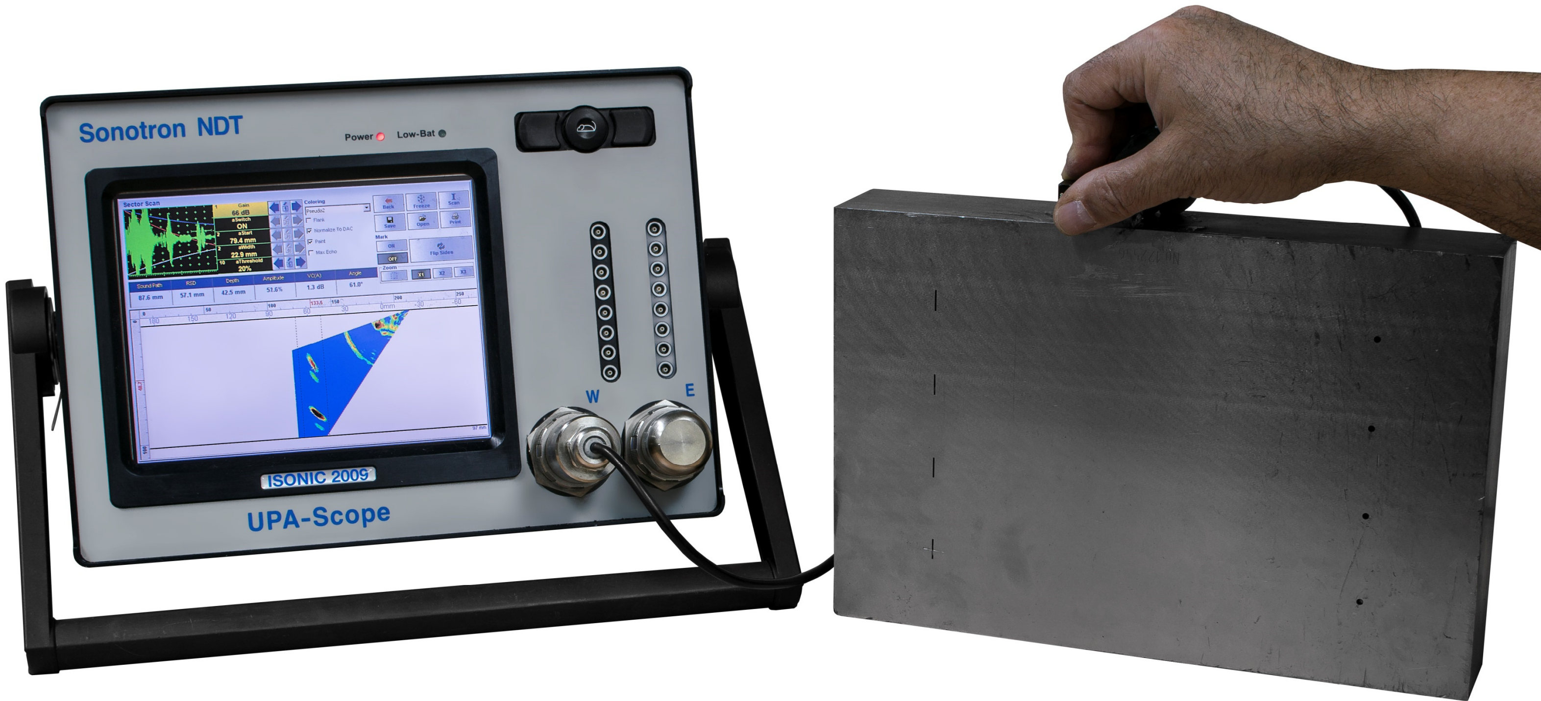
Longitudinal wave sector scan coverage of the heavy thickness calibration block with artificial vertical cracks – detection of upper / lower tip diffraction signals (one-side access reverse TOFD mode) – vertical line focusing
