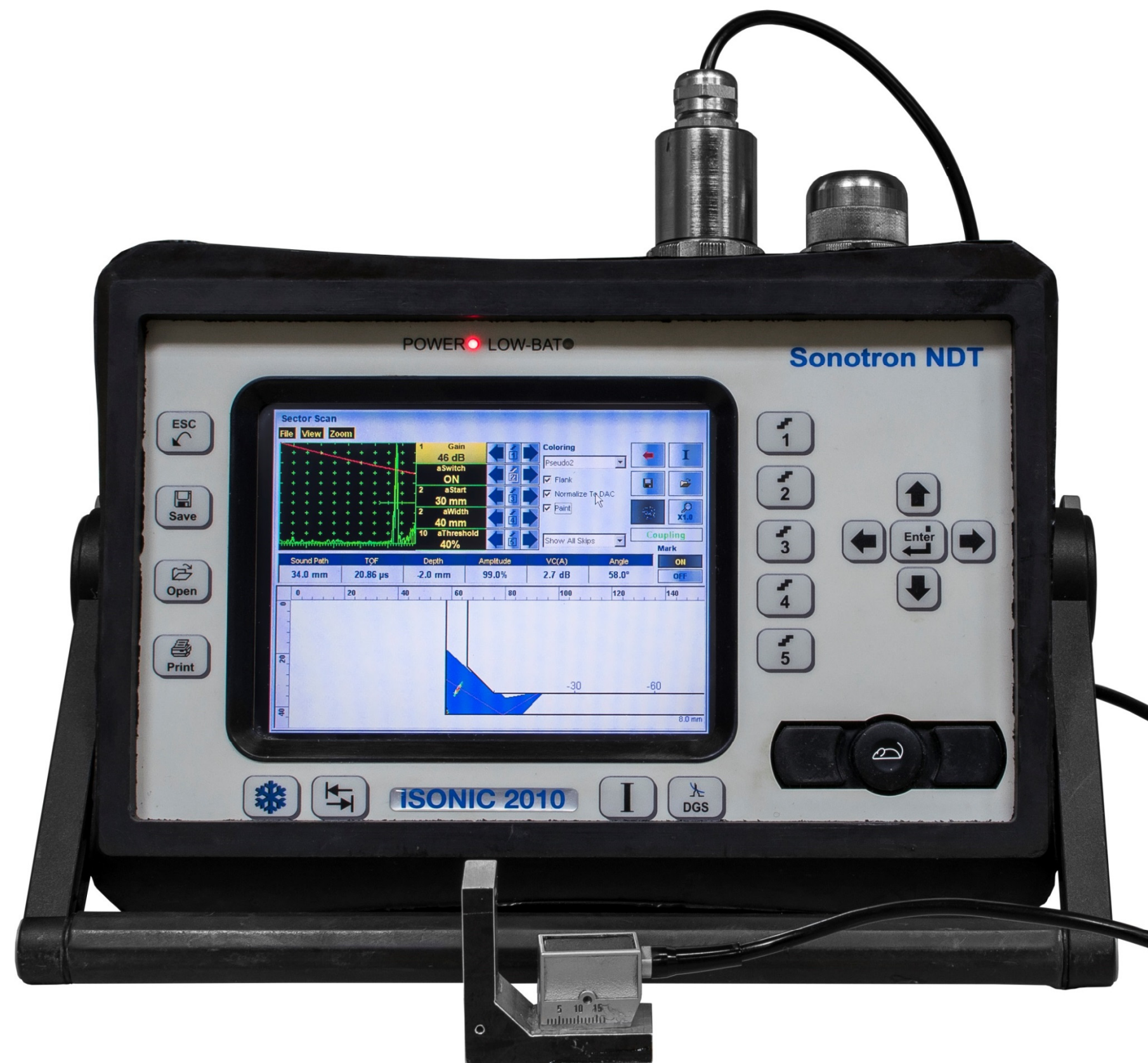
Shear wave inspection of the corner weld (calibration / performance demonstration block)
