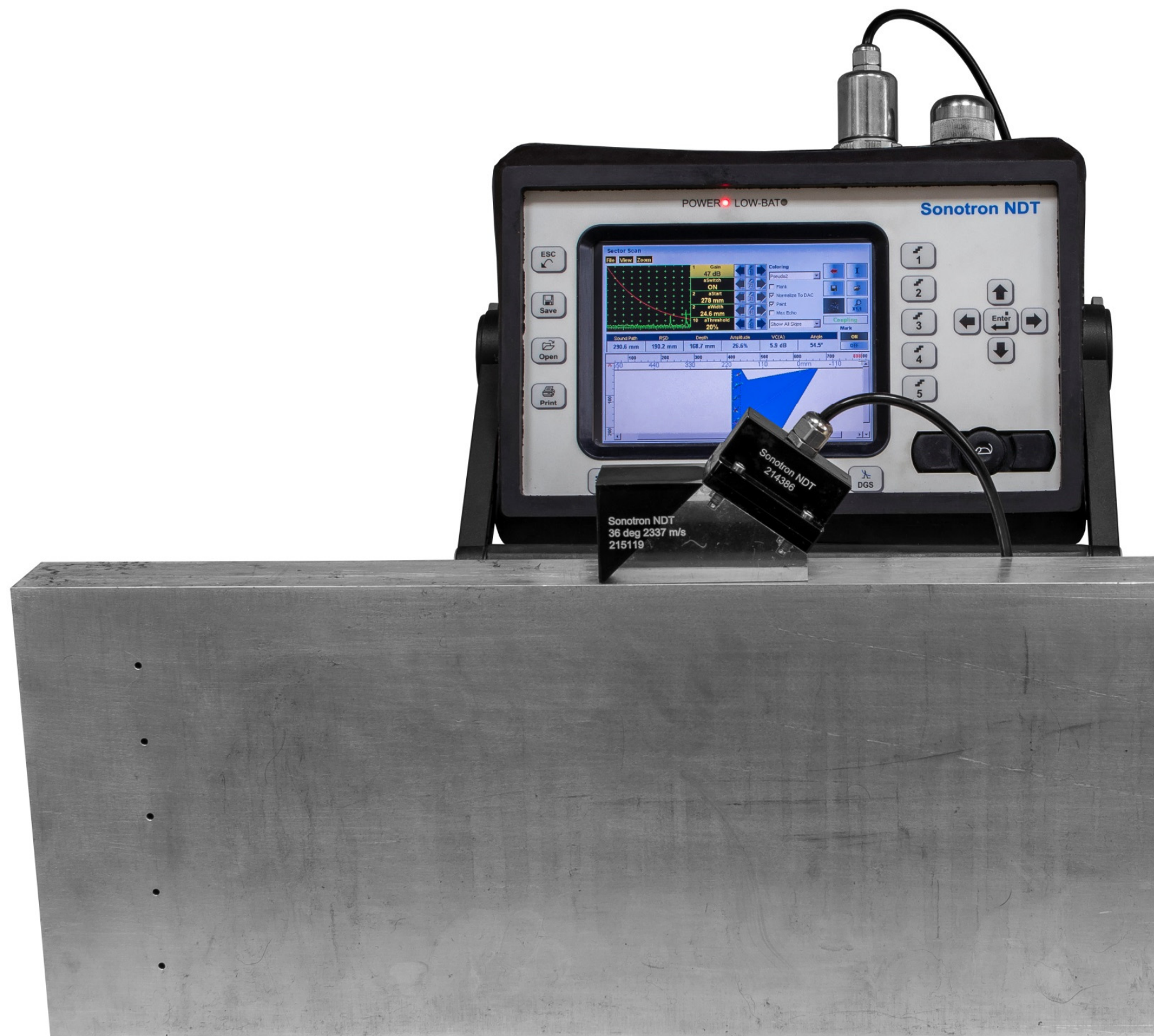
Combined half- and full skip inspection of 200 mm thick calibration block
