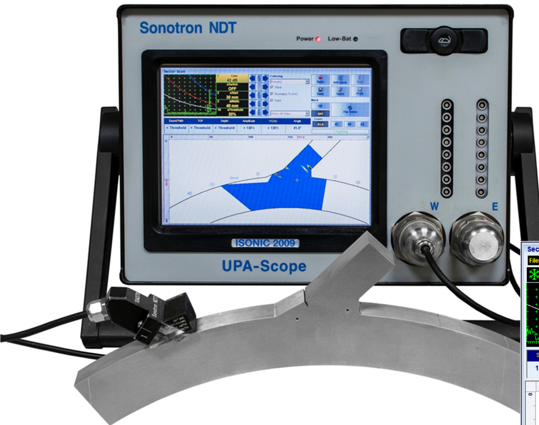
Shear wave inspection of the TKY weld – probe placement on the curved flange (performance demonstration block)
