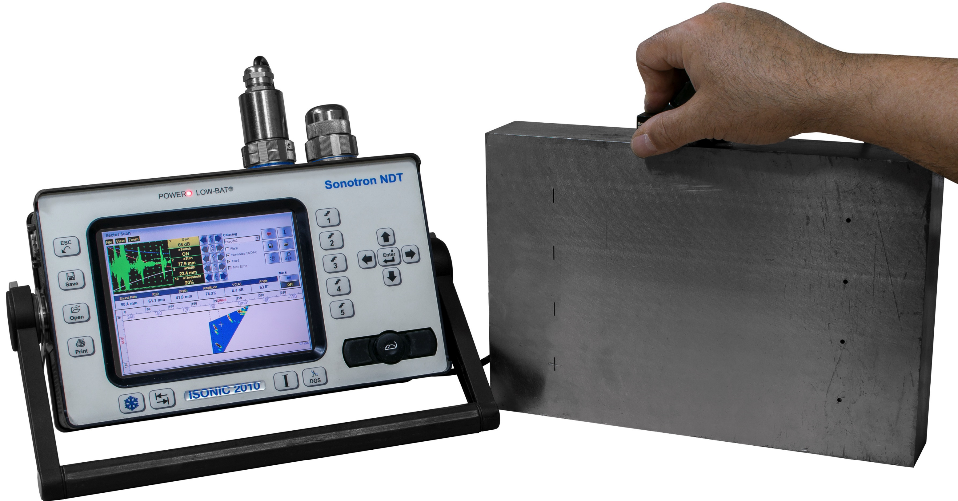
Longitudinal wave sector scan coverage of the heavy thickness calibration block with artificial vertical cracks – detection of upper / lower tip diffraction signals (one-side access reverse TOFD mode) – vertical line focusing
