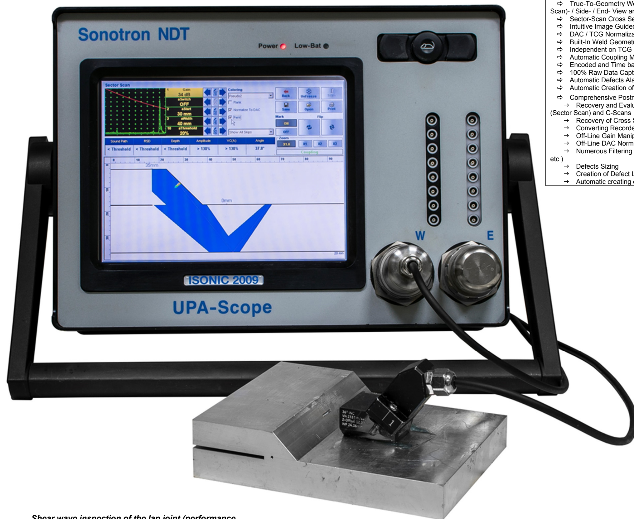
Shear wave inspection of the lap joint (performance demonstration block)
