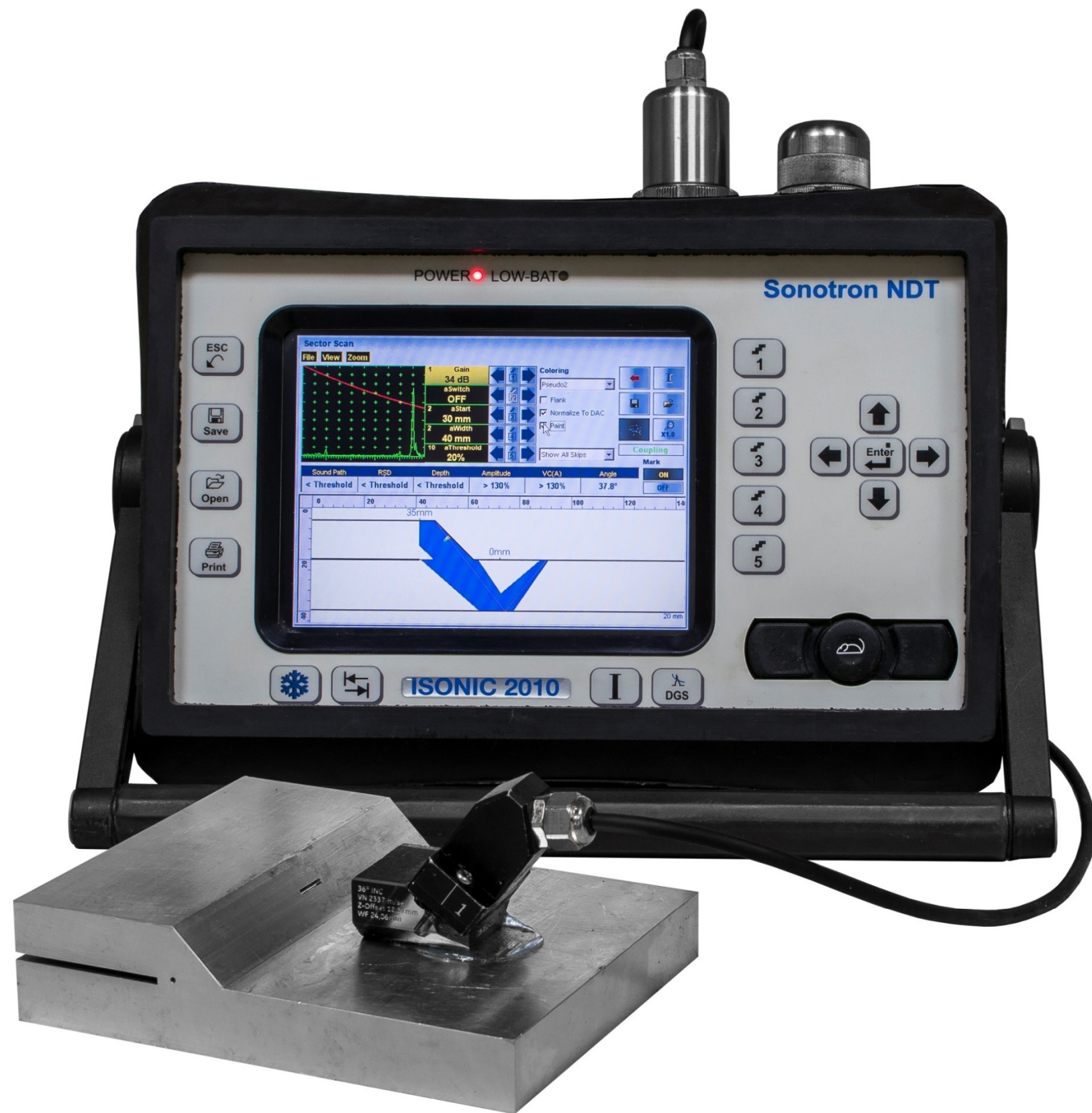
Shear wave inspection of the lap joint (performance demonstration block)
