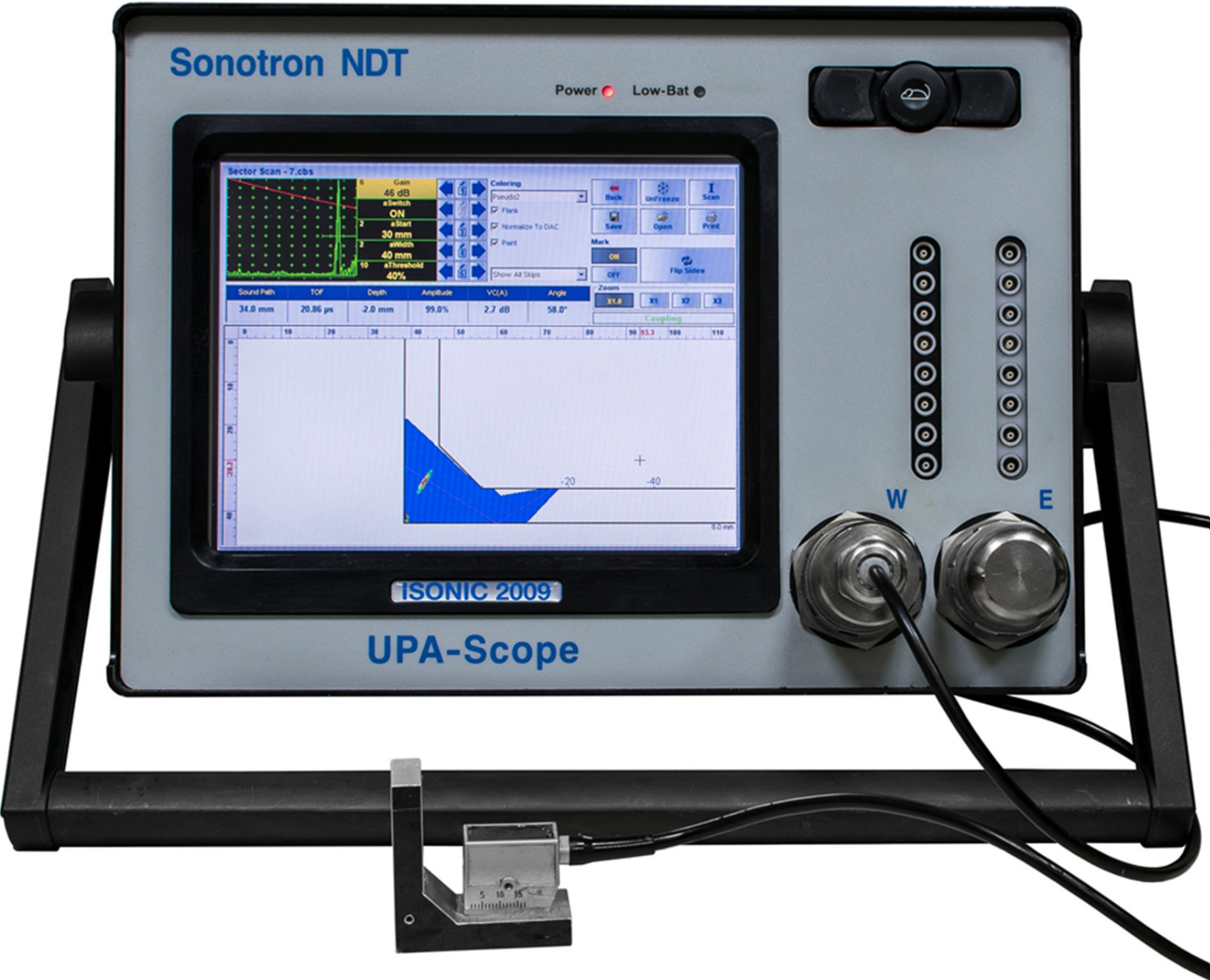
Shear wave inspection of the corner weld (calibration / performance demonstration block)
